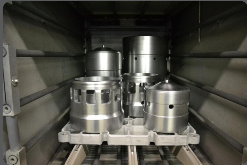
Vacuum hardening furnace with a load inside
