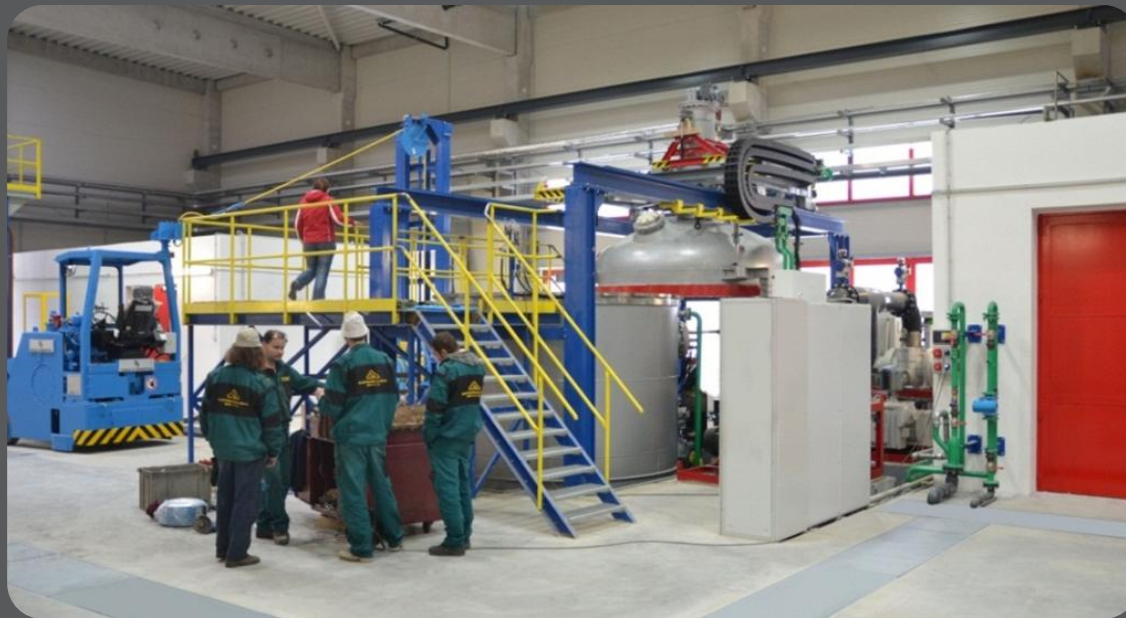
VIM furnace at COMTES FHT
