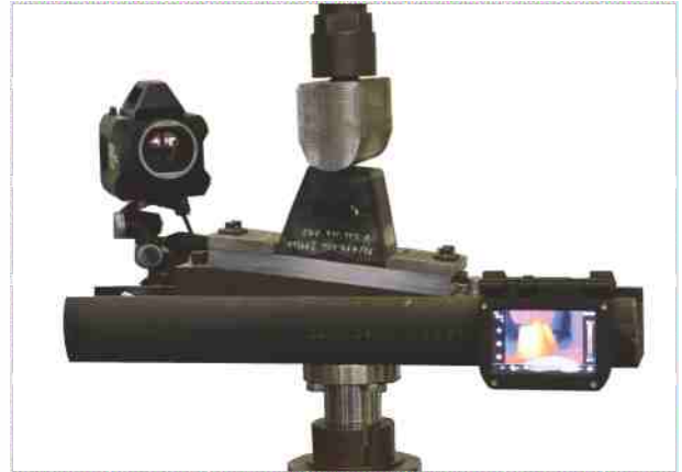
High-speed camera, max. 680,000 frames/s, resolution 1.0 MPx
