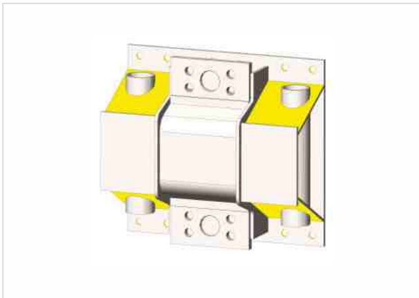
Fatigue testing segment
