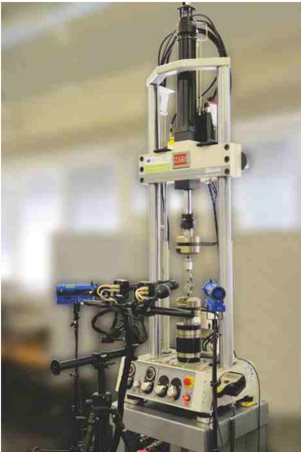
MTS Bionix servo-hydraulic biaxial testing machine, piston 1: 1 m/s 25 kN, 150°/s 250Nm, piston 2: 500 mm/s, 10 kN
