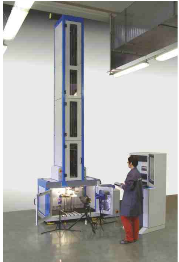
Drop tester tool energy 3000 J, max. loading speed 25 m/s
